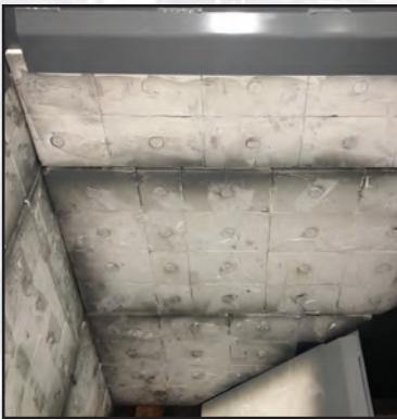
Head unit with optional ceramic tile liner for increased wear resistance.
