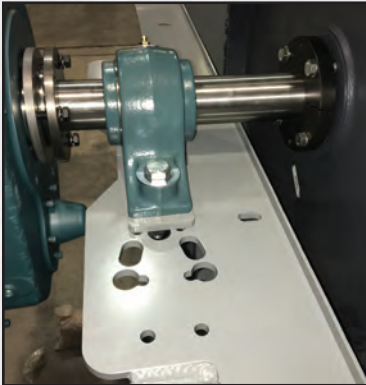
Tapered roller bearing mounted to laser-cut bearing plate and rain flange for weather-proof seal.
